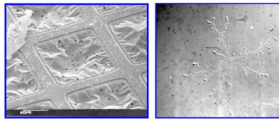
Photo 1: SEM micrograph of chromium film target of EVOs made by accretion from a surface run of electrons.
