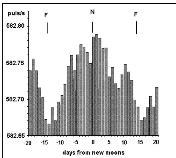
**Fig. 2.** Averaging over cycles of the synodic Lunar month of the count rate data for  $^{90}\text{Sr}$ - $^{90}\text{Y}$  beta source, as registered by G-M counter between April 2000 and March 2007. Averaging covers 87 cycles. N – new Moon, F - full Moon [6,7].
